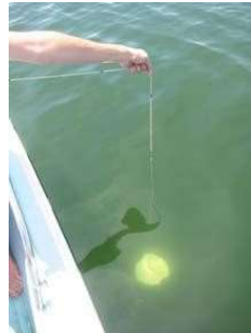
MEASUREMENT BEING TAKEN Note black measurement markings on tape attached to disk
